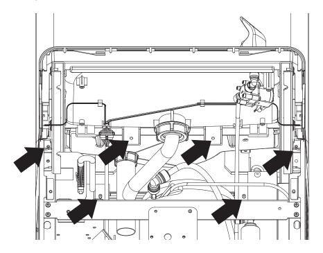
5TEP **6**  Remove the four screws that hold the basin to the steel frame. There are notches to help you locate them.
