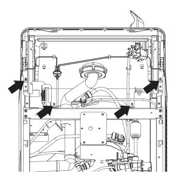
5TEP **28**  Replace the basin underside and secure it with four button-headed plastic screws. Replace the front panel and secure it with two flanged screws.
