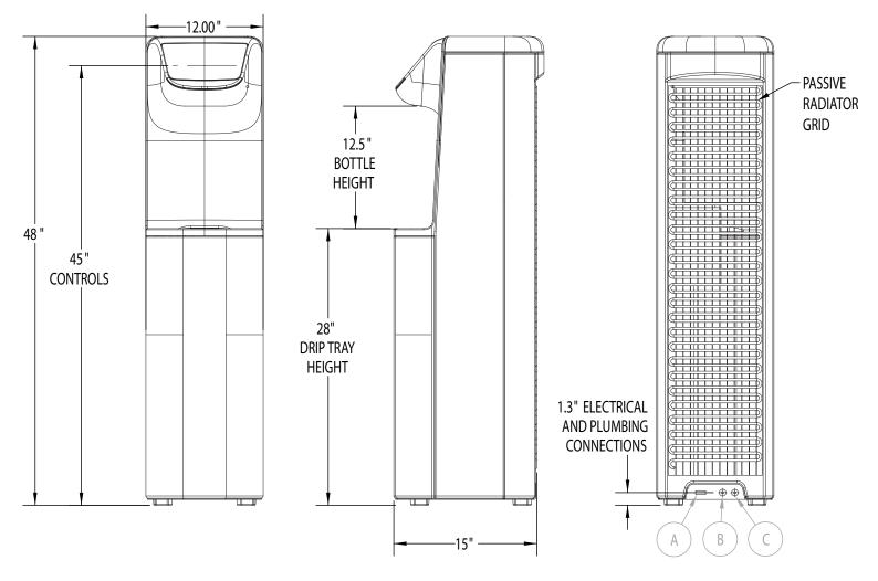
LEAVE AN ADDITIONAL 2" OF SPACE BEHIND THE UNIT FOR AIR FLOW AND ELECTRICAL AND PLUMBING CONNECTIONS
